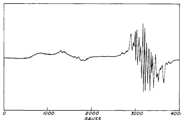
**Figure 3.** X-Band electron spin resonance spectrum of  $\text{PcMn}(\text{O}_2)$  dissolved in *N,N*-dimethylacetamide at approximately 4 K. Instrumental parameters: gain  $5 \times 10^3$ , frequency 9.150 GHz, pen response 0.016 s, power 0.2 mW, acquisition time 2 min, modulation amplitude 8 G, range 0–4000 G.
