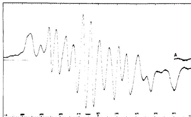
**Figure 2.** X-Band electron spin resonance spectrum of  $\text{PcMn}(\text{O}_2)$  dissolved in *N,N*-dimethylacetamide at approximately 4 K. The signal labeled A is offset 100 G and is, therefore, a continuation of the main spectrum. Instrumental parameters: gain  $8 \times 10^3$ , frequency 9.153 GHz, pen response 0.032 s, power 0.5 mW, acquisition time 4 min, modulation amplitude 4 G, range 2770–3870 G.
